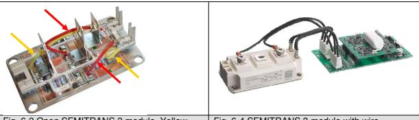
Fig. 6-3 Open SEMITRANS 3 module. Yellow and red wires are gate and emitter wires
