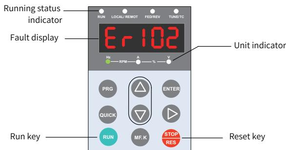
Figure 7-1 Fault display
