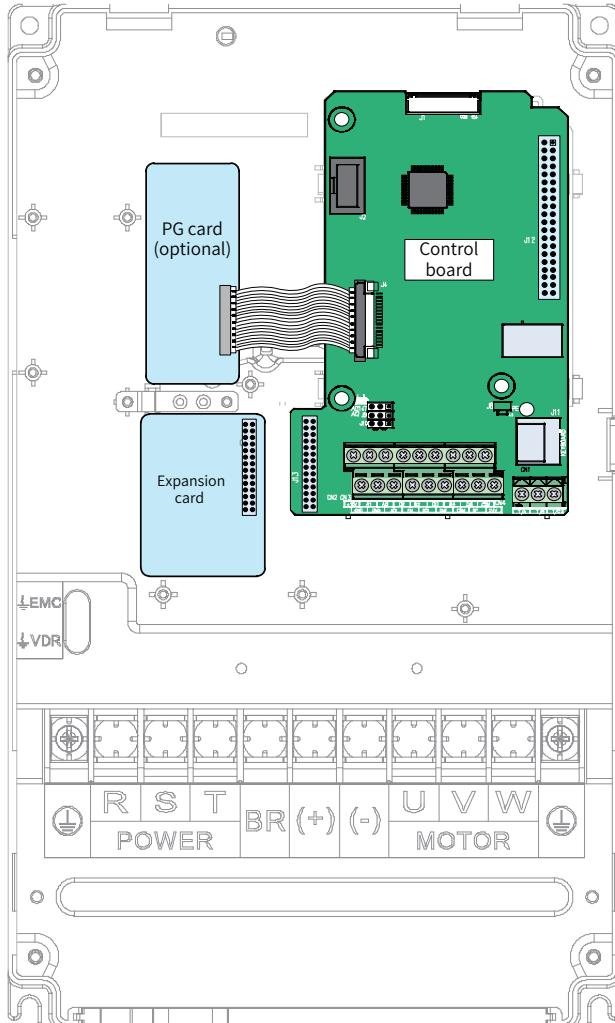
Figure 3-56 Installation position of the CS710 series AC drive control board
