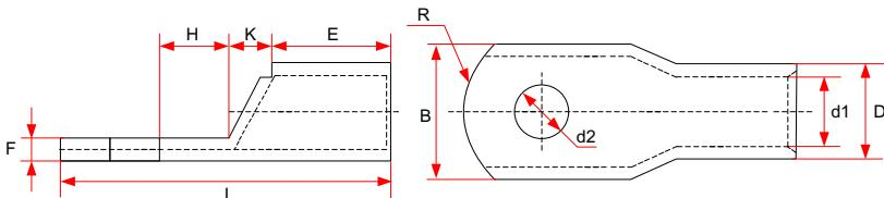
Figure 9-19 Dimensions of GTNR series cable lugs
