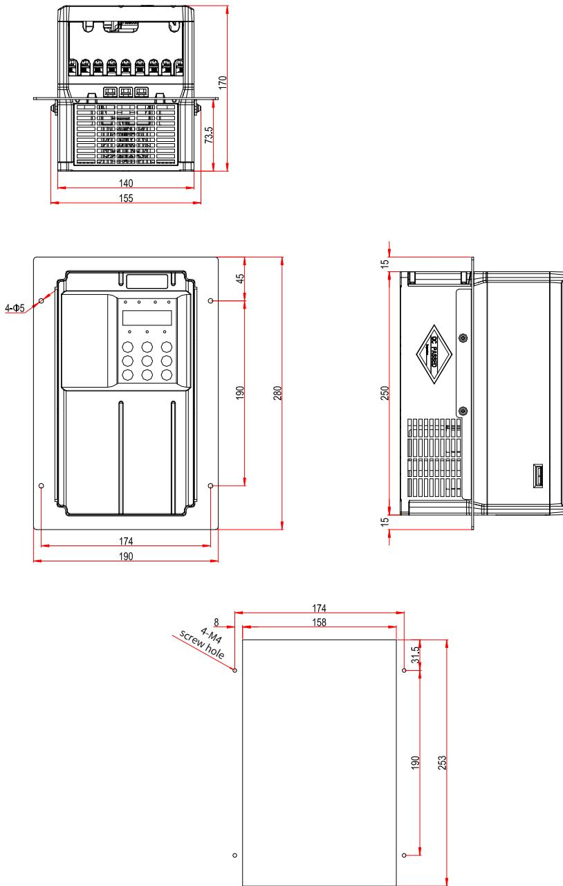
Figure 9-6 Through-hole mounting bracket and mounting hole dimensions for 7.5-11 kW AC drive models (mm)
