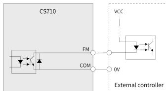
Figure 3-68 Wiring of high-speed DO FM
