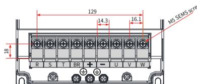
Figure 3-40 Dimensions of the main circuit terminals
