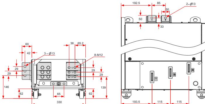
Figure 3-49 Dimensions of the main circuit terminals (CS710-4T250G/CS710-4T280G, without the output reactor) (mm)
