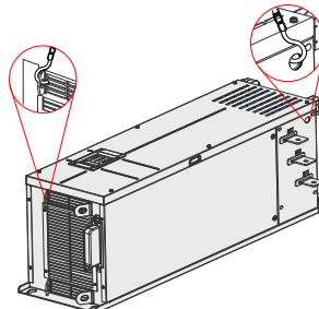
If the AC drive is placed vertically, do not apply force on two sides of the AC drive or place the AC drive on an inclined surface. The AC drive weighs almost 200 kg and may fall down if the slope exceeds 5°.
