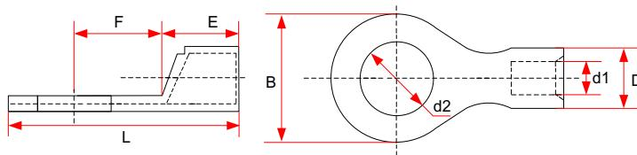
Figure 9-18 Dimensions of TNR series cable lugs
