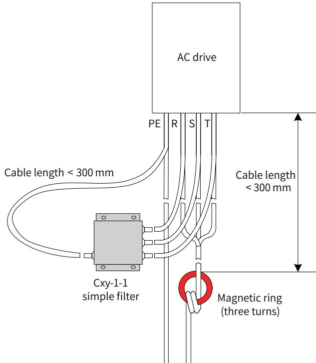
Figure 9-22 Installing a simple filter and magnetic ring on the input side
