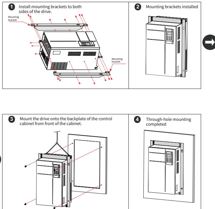
Figure 3-10 Through hole mounting of 45–160 kW models
