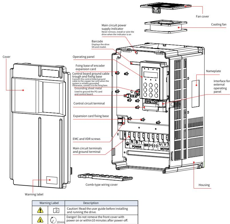
Figure 1-3 Components (three-phase 380–480 V, 18.5–37 kW)
