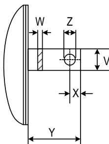
Figure B-7 Dimensions of grounding copper busbar
