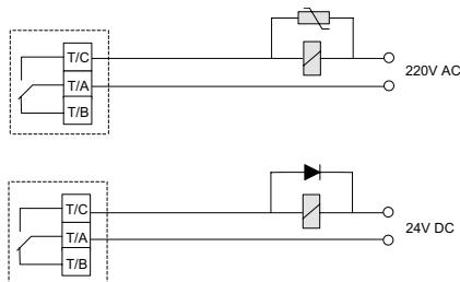
Figure 3-69 Anti-interference treatment for the relay output terminal
