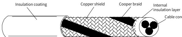
Figure B-15 Shield of a shielded cable
