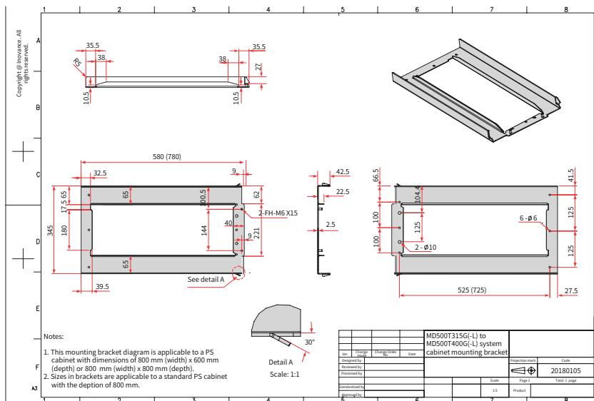
Figure 9-17 Dimensions of the mounting bracket for 315–400 kW AC drives (standard configuration) (mm)
