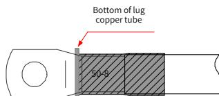
Figure 3-36 Heat-shrink tubing for cable conductor
