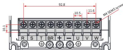
Figure 3-38 Dimensions of the main circuit terminals (CS710-4T0.4GB to CS710-4T5.5GB, three phase 380–480 V) (mm)
