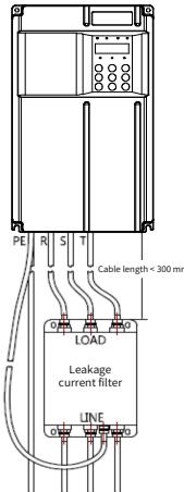
Figure B-13 Simple filter installation
