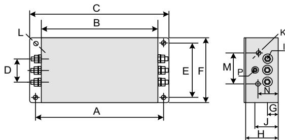
Figure B-10 Dimensions of JIANLI filters (50 A to 200 A)
