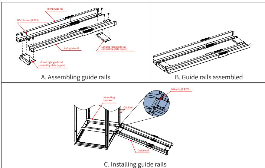
Figure 3-18 Mounting guide rails on the cabinet
