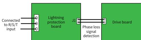
Figure 8-2 Connection between the lightning protection board and driver board for the AC drive of 45 kW and above
