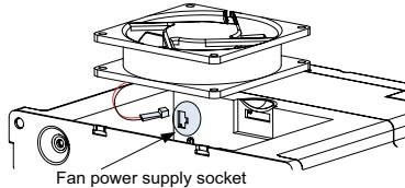
3. Install the fan into the AC drive and ensure that the four fixed holes are aligned with the positioning pins.
