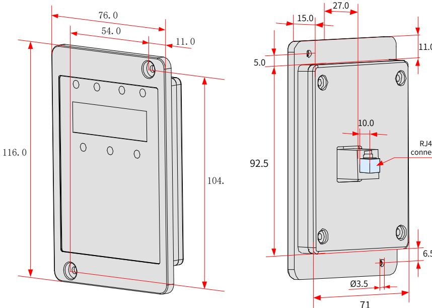
Figure 9-23 Dimensions of the external operating panel (mm)
