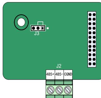
Figure 10-8 Terminal layout on MD38TX1
