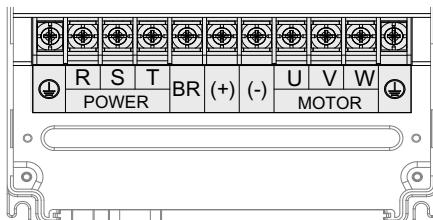
Figure 3-28 Layout of main circuit terminals of 18.5–160 kW models
