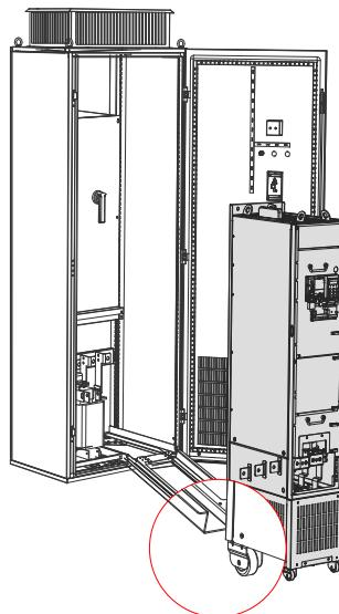
Figure 3-19 Aligning the AC drive casters with the guide rails
