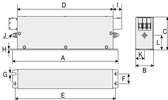
Figure B-4 Dimensions of FN 3258 series filters (50 A to 180 A)
