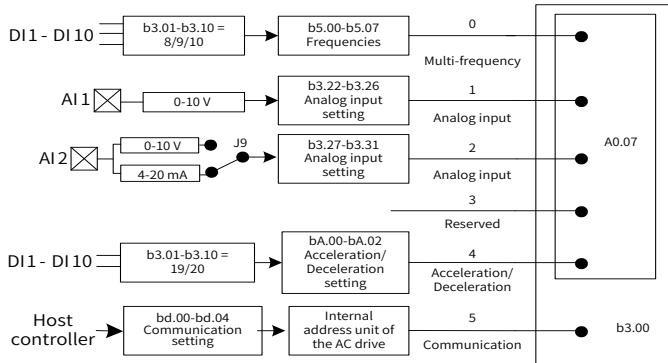
Figure 5-5 Frequency reference source selection
