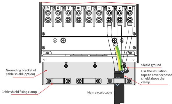
Figure 3-33 Shield wiring
