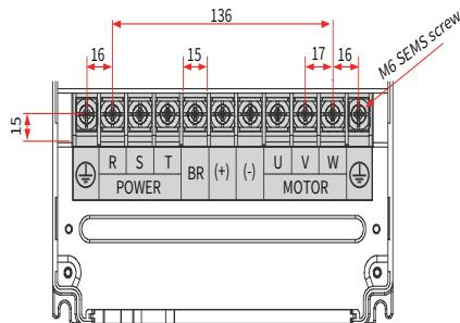
Figure 3-41 Dimensions of the main circuit terminals
