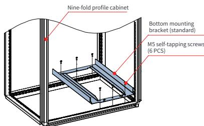
Figure 3-17 Installing the bottom mounting bracket
