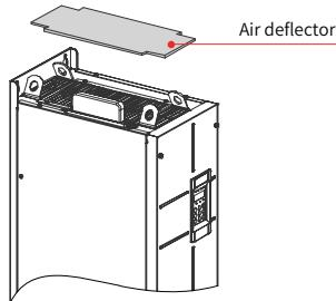
Use the eye bolt on the top of the AC drive to lift or move the drive. To lift an AC drive that is lying flat, use the lift fittings on the top and bottom of the drive. Do not apply force on the positive and negative bus terminals.
