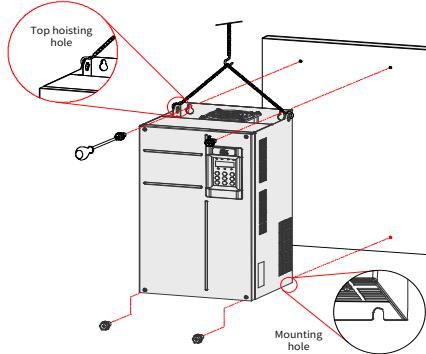
Figure 3-8 Backplate mounting for 45–160 kW models
