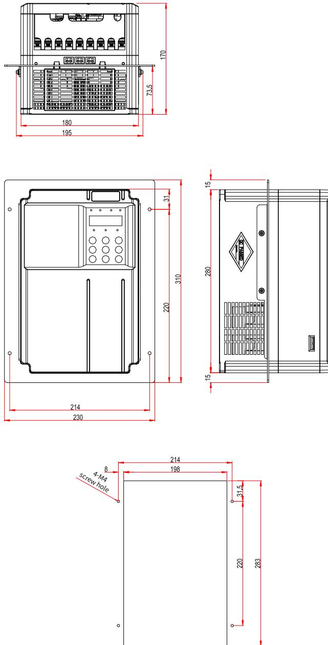
Figure 9-7 Through-hole mounting bracket and mounting hole dimensions for 15 kW AC drive models (mm)
