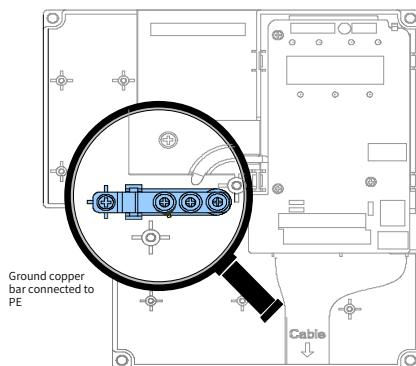
CS710 has a grounding structure. After a PG card is installed, the PE terminal of the PG card can be connected to the AC drive internally. When connecting an encoder, connect the shield of the signal cable to the PE terminal of the PG card to complete the shield grounding.
