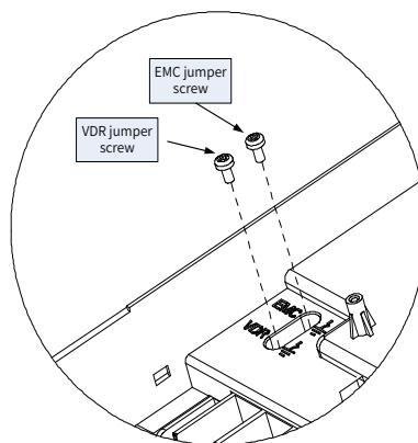
Figure B-18 EMC and VDR jumper screws
