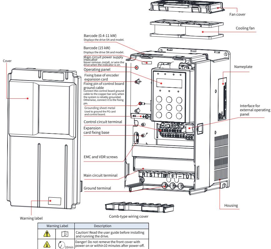
Figure 1-2 Components (three-phase 380–480 V, 0.4–15 kW)
