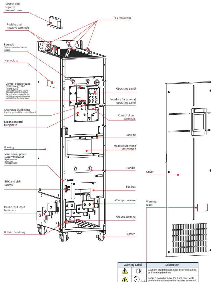
Figure 1-5 Components (three-phase 380–480 V, 200–400 kW)
