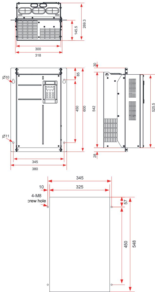
Figure 9-10 Through-hole mounting bracket and mounting hole dimensions for 45–55 kW AC drive models (mm)
