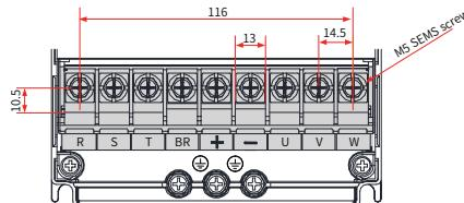
Figure 3-39 Dimensions of the main circuit terminals
