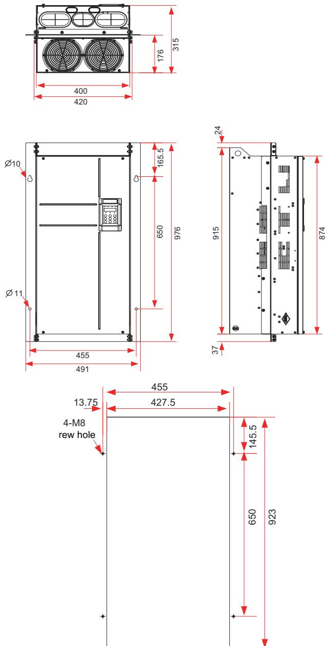
Figure 9-12 Through-hole mounting bracket and mounting hole dimensions for 132-160 kW AC drive models (mm)
