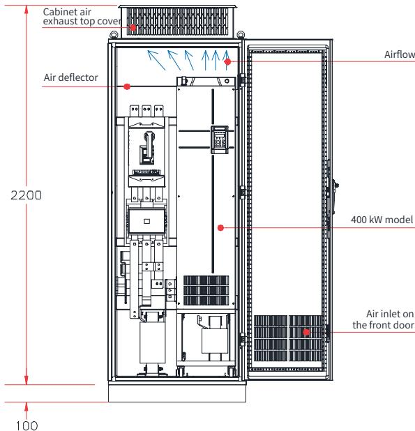
Figure 3-11 Self-ventilated cabinet (without fans on the top)
