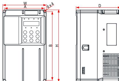
Figure 9-1 Outline dimensions and installation dimensions of 0.4–15 kW AC drive models
