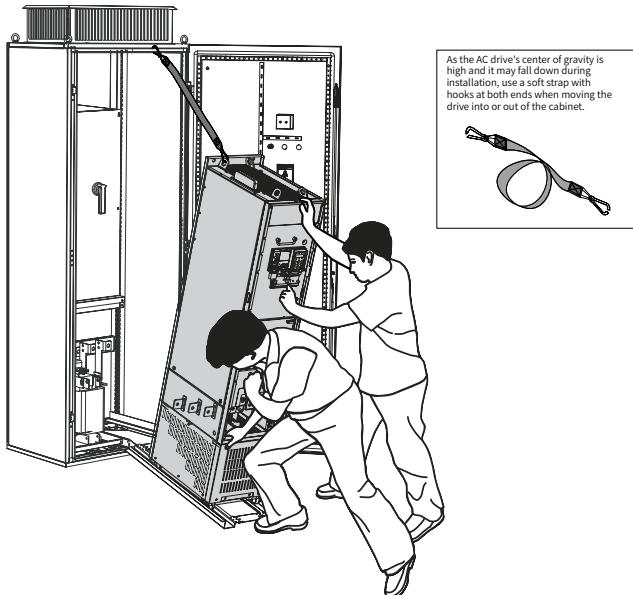
Figure 3-20 Pushing the AC drive slowly into the cabinet
