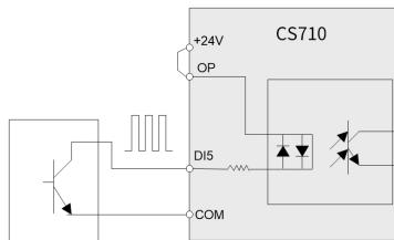
Figure 3-66 High-speed pulse input
