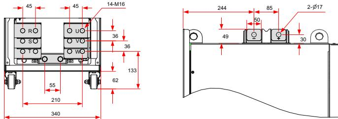
Figure 3-54 Dimensions of the main circuit terminals (CS710-4T315G to CS710-4T400G, without the side copper busbars or output reactor) (mm)
