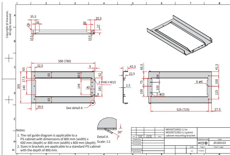
Figure 9-15 Dimensions of the mounting bracket for 200–220 kW AC drives (standard configuration) (mm)
