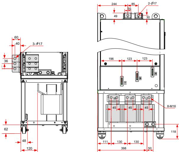
Figure 3-53 Dimensions of the main circuit terminals (CS710-4T315G to CS710-4T400G, with the output reactor) (mm)
