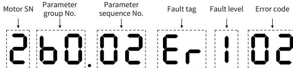
Figure 4-2 Example of the LED display
