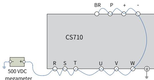
Figure 8-1 Insulation test on the main circuit
