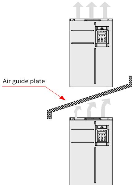
Figure 3-5 Installation of drives in dual-row
