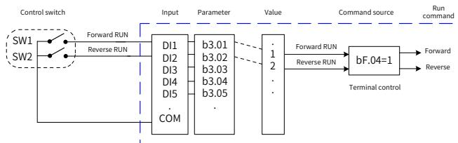
Figure 5-2 Example of AC drive control using terminals
