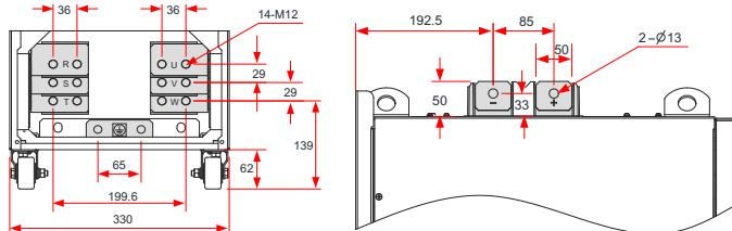
Figure 3-51 Dimensions of the main circuit terminals (CS710-4T250G/CS710-4T280G, without the side copper busbars or output reactor) (mm)
