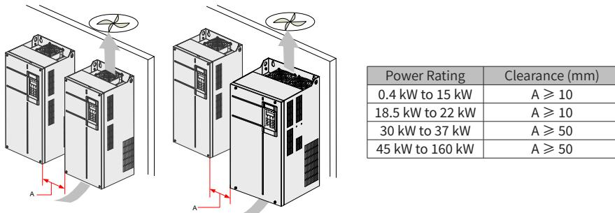
Figure 3-4 Installation clearance for side-by-side installation of multiple drives
