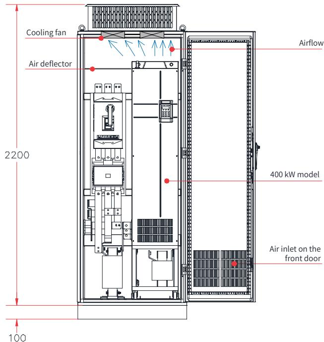
Figure 3-12 Force-ventilated cabinet (with top-mounted fans) (mm)
