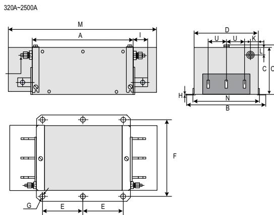
Figure B-6 Dimensions of FN 3359 series filters (320 A to 2500 A)
