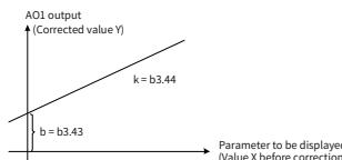
Figure 5-8 Output characteristic curve of AO1
