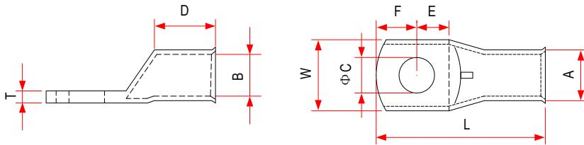
Figure 9-20 Dimensions of BC series cable lugs
