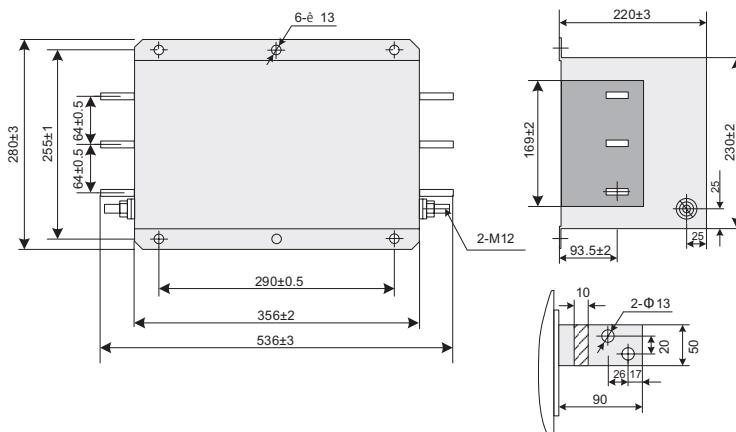
Figure B-12 Dimensions of JIANLI filters (1000 A) (mm)
