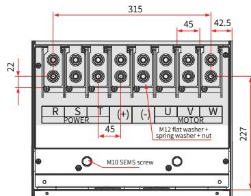
Figure 3-45 Dimensions of the main circuit terminals (CS710-4T132G/CS710-4T160G) (mm)
