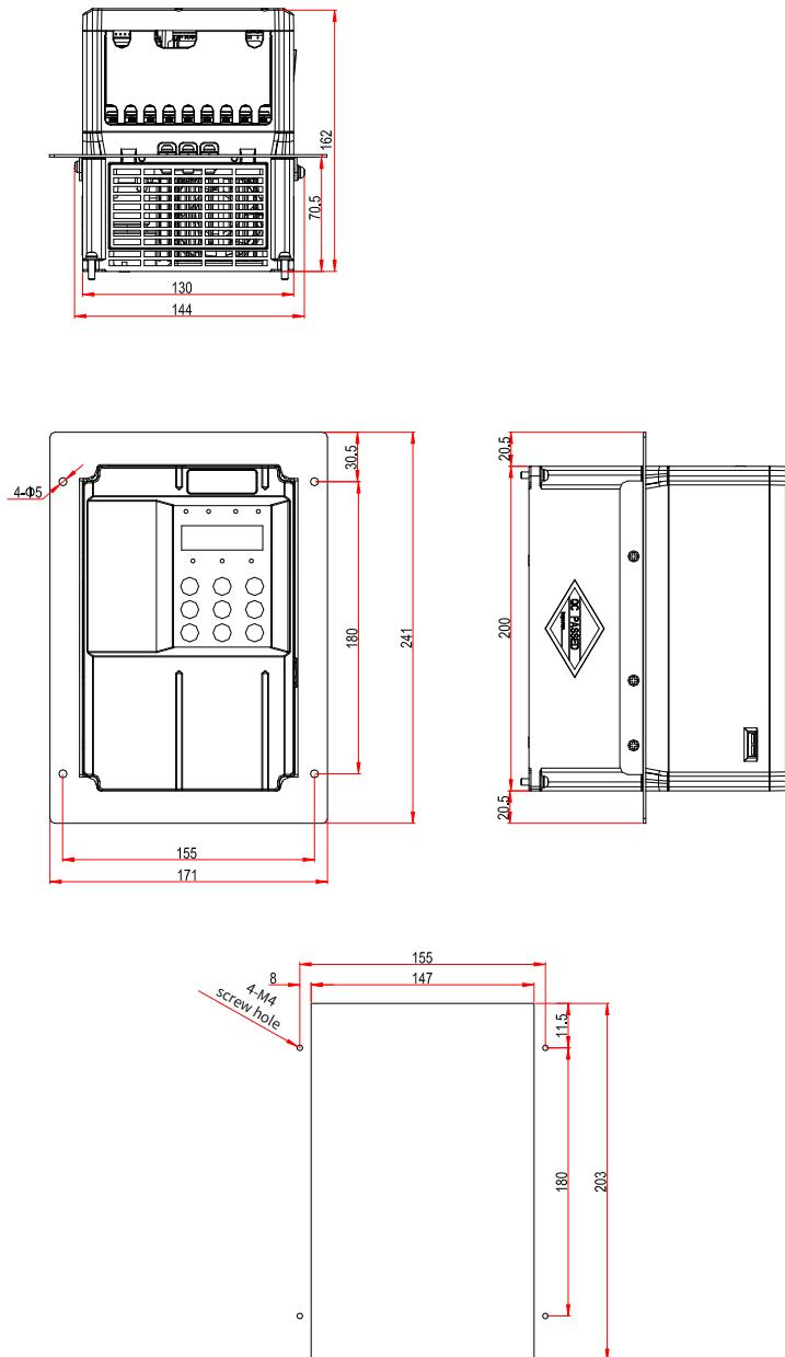
Figure 9-5 Through-hole mounting bracket and mounting hole dimensions for 3.7-5.5 kW AC drive models (mm)
