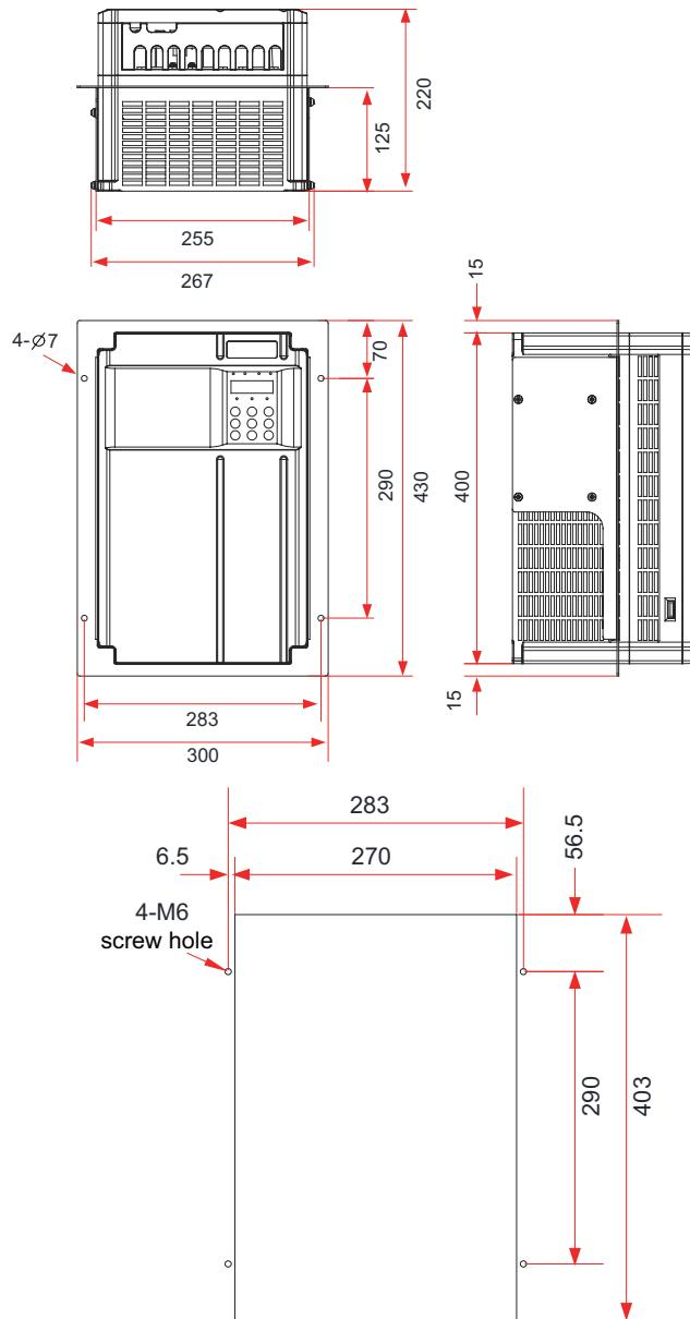
Figure 9-9 Through-hole mounting bracket and mounting hole dimensions for 30-37 kW AC drive models (mm)
