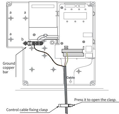
Figure 3-61 Grounding the shield of AI cable
