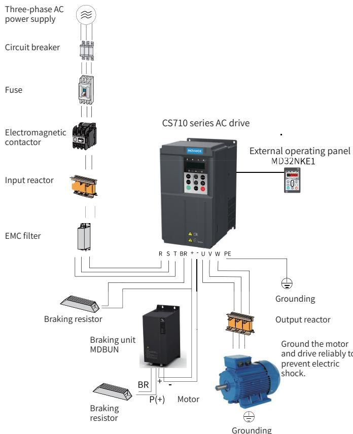
Figure 2-1 CS710 series AC drive system composition
