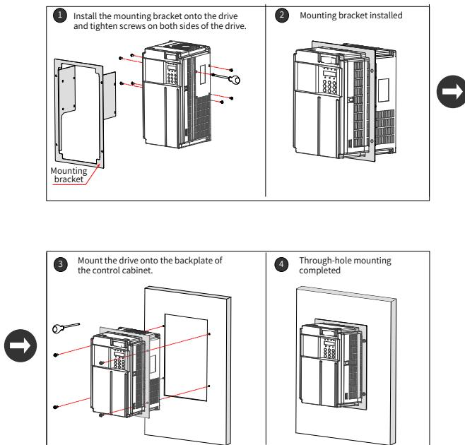
Figure 3-9 Through hole mounting of 0.4-37 kW models
