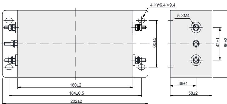
Figure B-9 Dimensions of JIANLI filters (20 A to 30 A)
