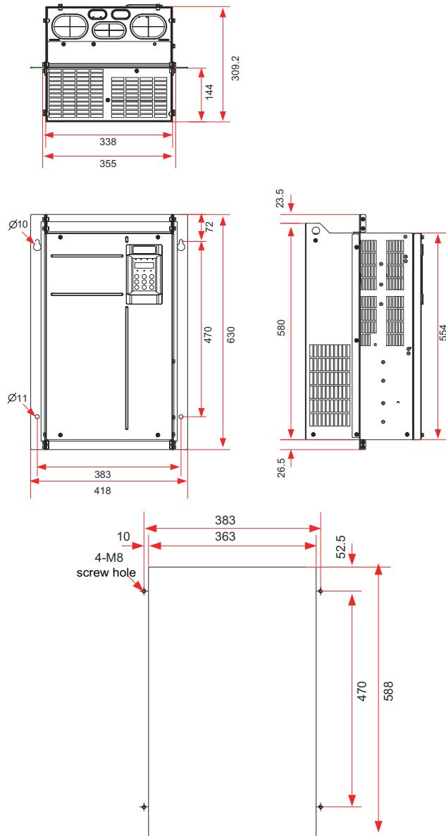
Figure 9-11 Through-hole mounting bracket and mounting hole dimensions for 75–110 kW AC drive models (mm)
