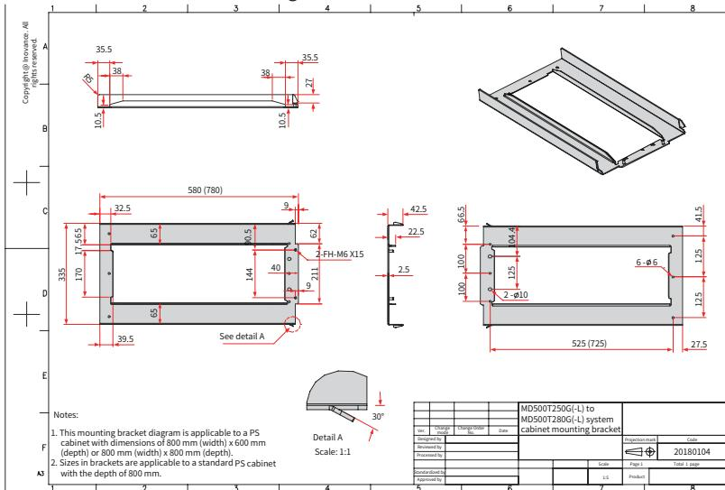
Figure 9-16 Dimensions of the mounting bracket for 250–280 kW AC drives (standard configuration) (mm)
