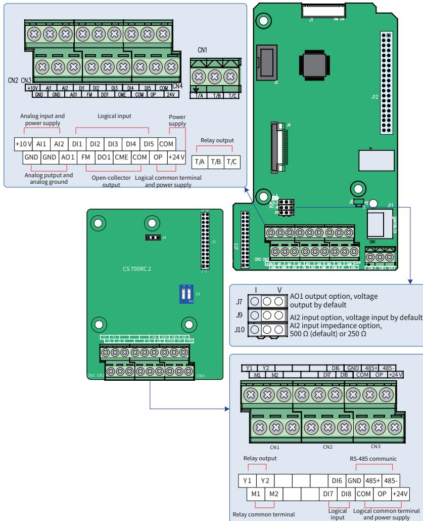
Figure 3-57 Control circuit terminal layout
