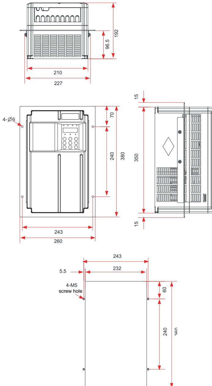
Figure 9-8 Through-hole mounting bracket and mounting hole dimensions for 18.5–22 kW AC drive models (mm)
