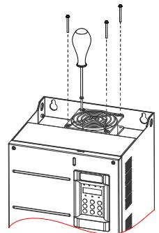
Remove the fan and fan cover from the AC drive.
