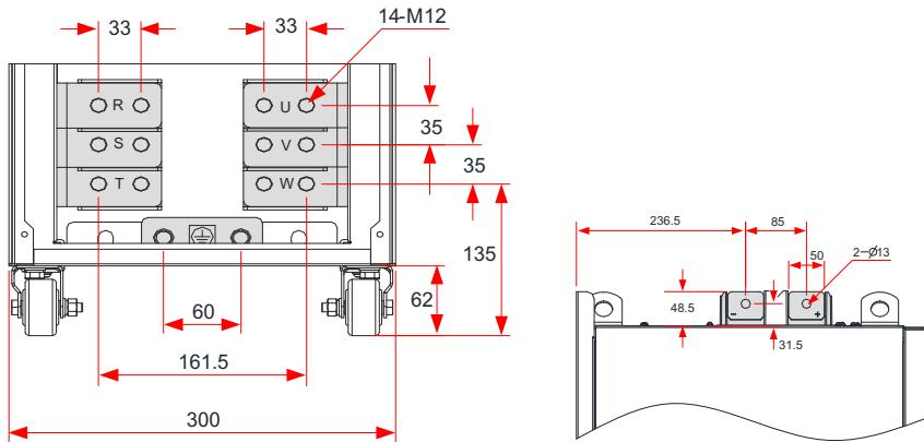
Figure 3-48 Dimensions of the main circuit terminals (CS710-4T200G, CS710-4T220G, without the side copper busbars or output reactor) (mm)
