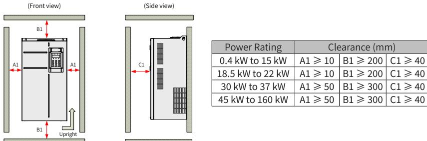
Figure 3-2 Installation clearance for a single drive (three-phase 380–480 V, 0.4–160 kW)
