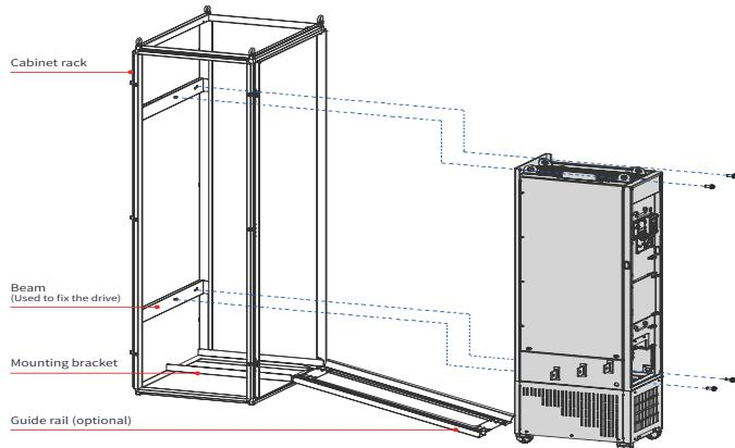
Figure 3-22 Fixing the AC drive to the fixing beam by using the four mounting holes on the back of the AC drive
