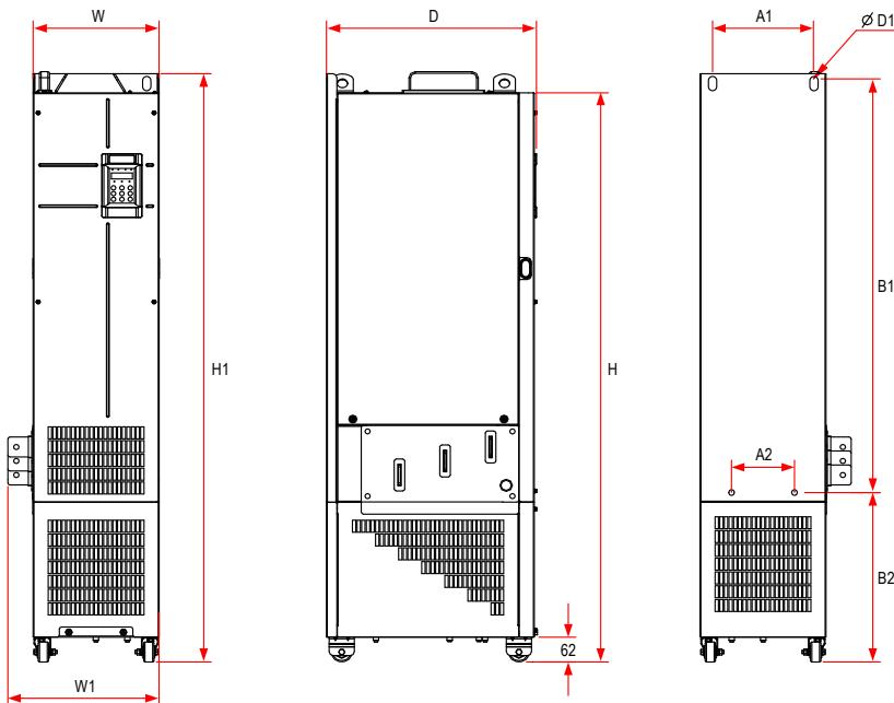
Figure 9-14 Outline dimensions and installation dimensions of 200–400 kW AC drive models (with the reactor base)
