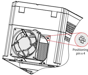
**Installing the fan (1.5–37 kW)**
