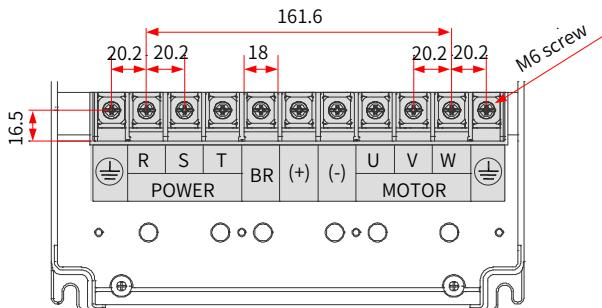
Figure 3-42 Dimensions of the main circuit terminals
