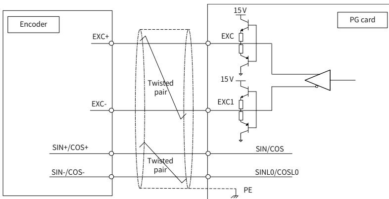
Figure 10-11 interface circuit on MD38PG4
