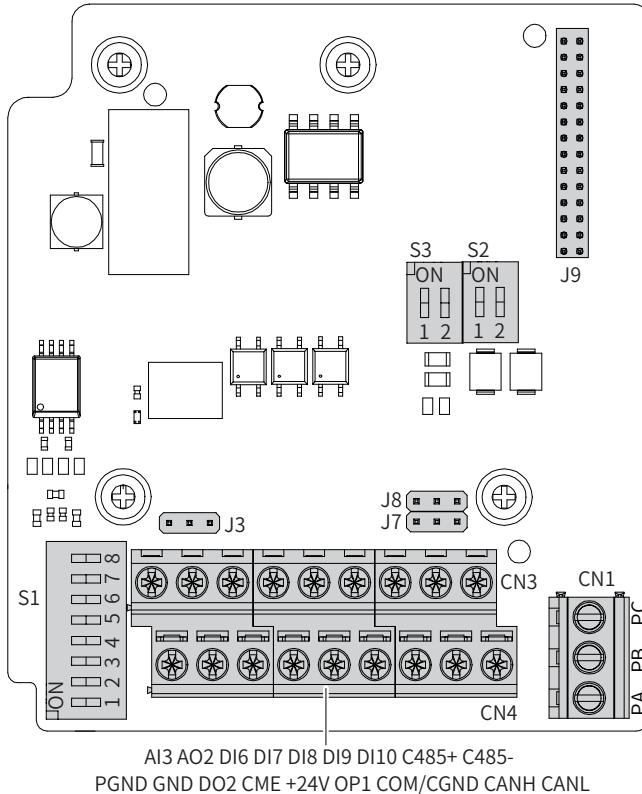
Figure 10-1 Terminal layout on MD38IO1
