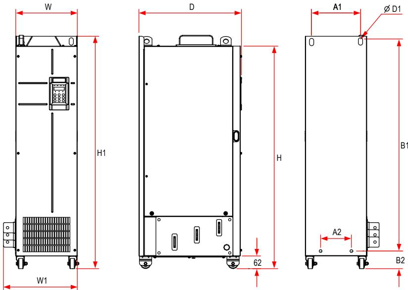
Figure 9-13 Outline dimensions and installation dimensions of 200–400 kW AC drive models (without the reactor base)
