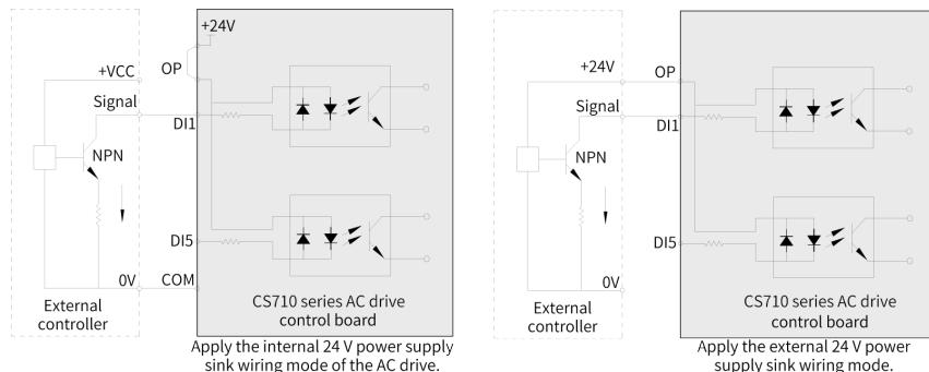
Figure 3-63 Sink wiring
