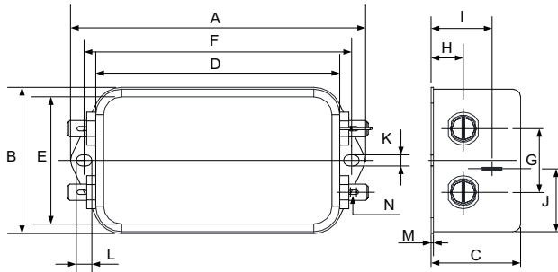
Figure B-2 Dimensions of FN 2090 series filters (8 A to 12 A)
