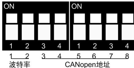
Figure 10-7 MD38CAN2 DIP switches
