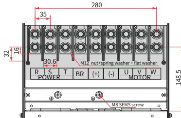
Figure 3-44 Dimensions of the main circuit terminals
