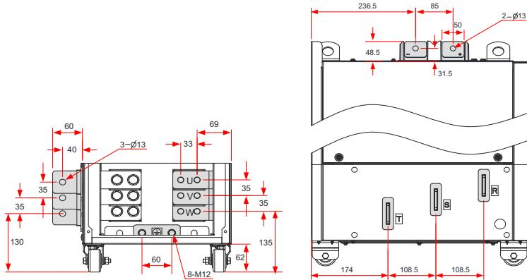
Figure 3-46 Dimensions of the main circuit terminals
