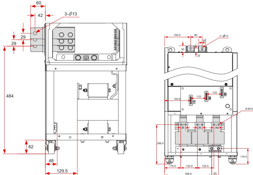
Figure 3-50 Dimensions of the main circuit terminals (CS710-4T250G/CS710-4T280G, with the output reactor) (mm)
