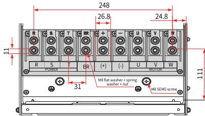
Figure 3-43 Dimensions of the main circuit terminals
