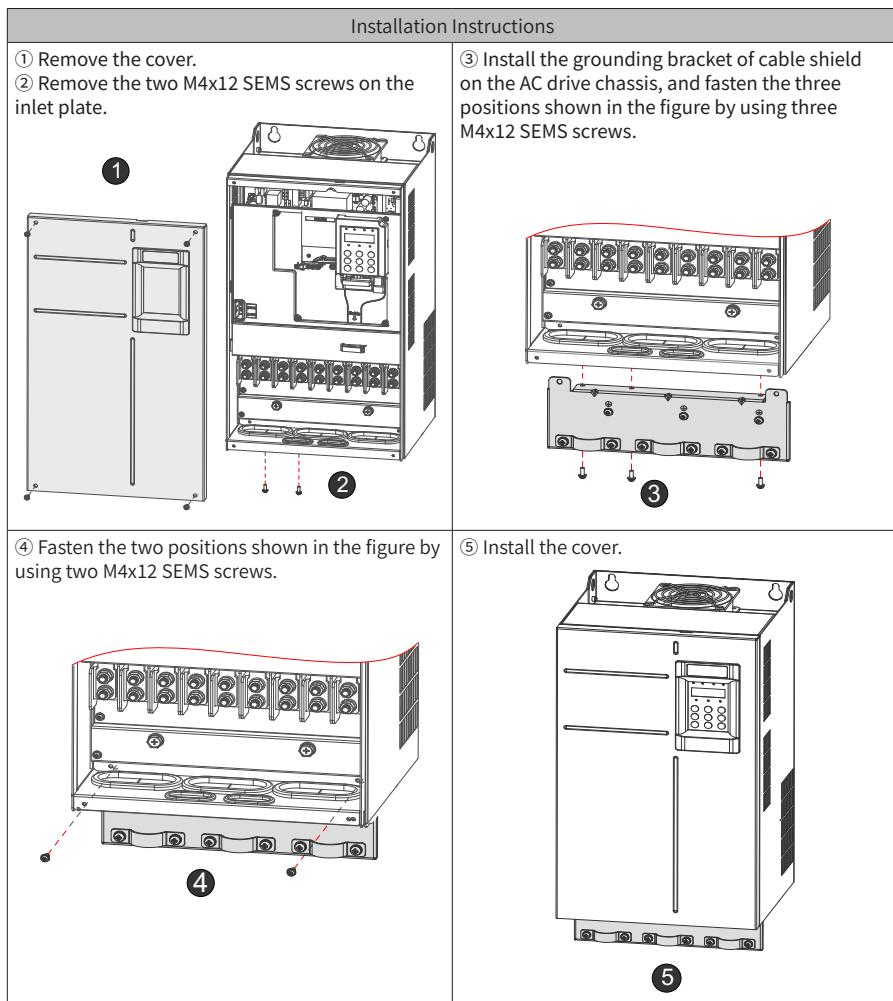
Figure 3-34 Installation of the grounding bracket of cable shield
