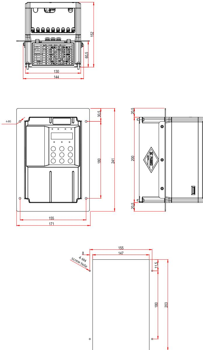
Figure 9-4 Through-hole mounting bracket and mounting hole dimensions for 0.4–3.0 kW AC drive models (mm)
