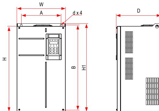
Figure 9-3 Outline dimensions and installation dimensions of 45-160 kW AC drive models
