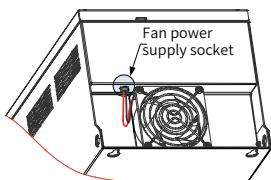
Remove the four screws from the fan cover using a screwdriver.
