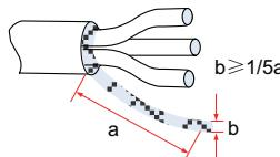
Figure 3-35 Drain wire of the motor cable shield
