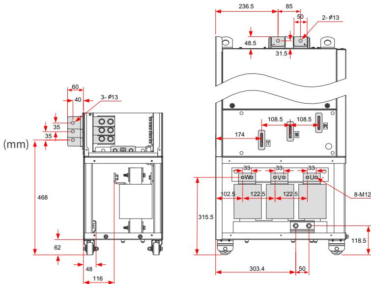
Figure 3-47 Dimensions of the main circuit terminals (CS710-4T200G/CS710-4T220G, with the output reactor) (mm)
