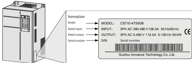
Figure 1-1 Nameplate and model number
