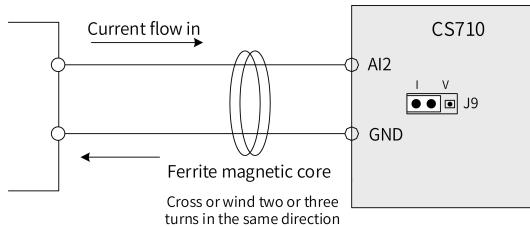
Figure 3-62 Wiring of AI2
