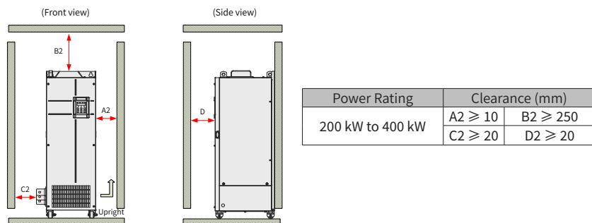
Figure 3-3 Installation clearance for a single drive [three-phase 380–480 V, 200–400 kW]
