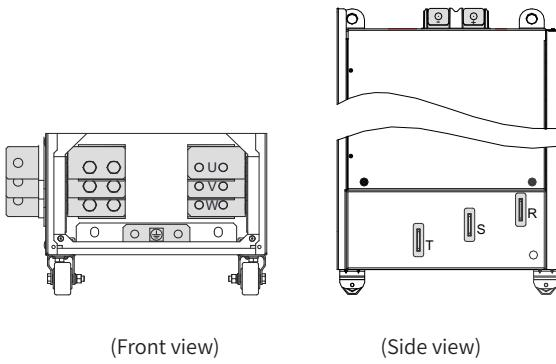
Figure 3-29 Layout of main circuit terminals of 200–400 kW models
