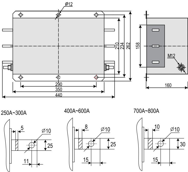
Figure B-11 Dimensions of JIANLI filters (250 A to 800 A) (mm)
