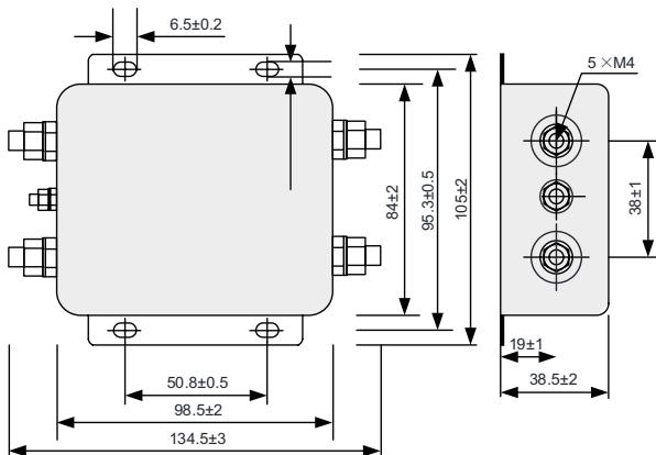
Figure B-8 Dimensions of JIANLI filters (10 A)
