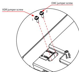
Figure 3-37 Positions of VDR and EMC ground jumpers
