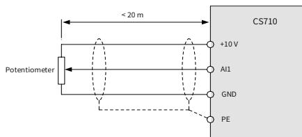
Figure 3-60 Wiring of AI1
