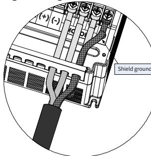
Figure B-16 Grounding of a shielded cable
