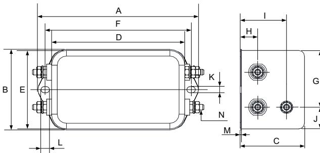
Figure B-3 Dimensions of FN 2090 series filters (20 A to 30 A)
