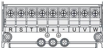
Figure 3-27 Layout of main circuit terminals of 0.4–15 kW models
