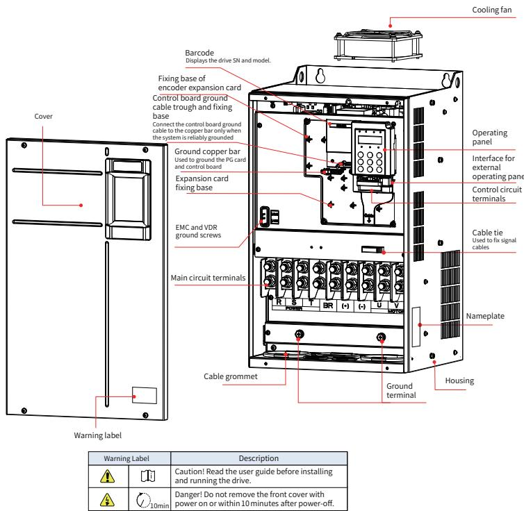
Figure 1-4 Components (three-phase 380–480 V, 45–160 kW)
