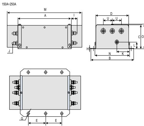
Figure B-5 Dimensions of FN 3359 series filters (150 A to 250 A)
