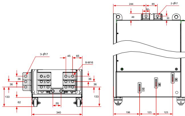
Figure 3-52 Dimensions of the main circuit terminals (CS710-4T315G to CS710-4T400G, without the output reactor) (mm)
