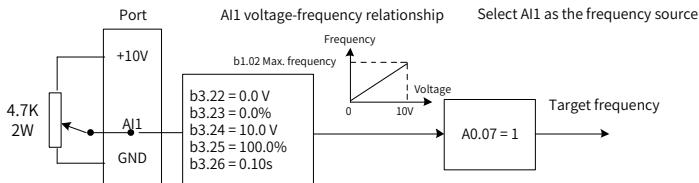
Figure 5-7 Using the AI to set frequency reference
