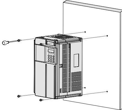
Figure 3-7 Backplate mounting for 0.4–37 kW models
