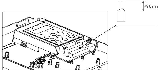
Figure 3-70 Requirements on the tubular terminal of a control cable
