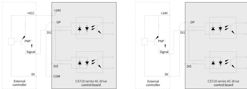
Figure 3-65 Source wiring
