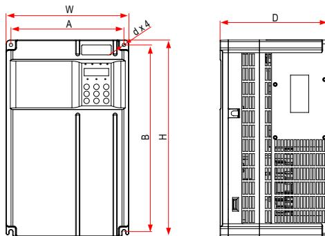
Figure 9-2 Outline dimensions and installation dimensions of 18.5-37 kW AC drive models
