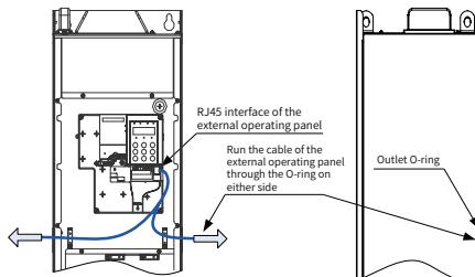
Figure 3-71 Wiring for connecting the external operating panel
