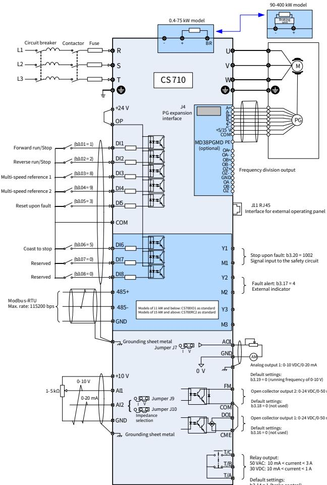
Figure 3-26 Typical wiring of three-phase 380–480 V drive
