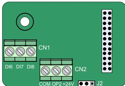
Figure 10-2 Terminal layout on MD38IO2
