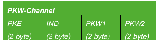
Fig. 1.2: Structure of PKW telegram for C-Line, LeviOne and ServoOne
