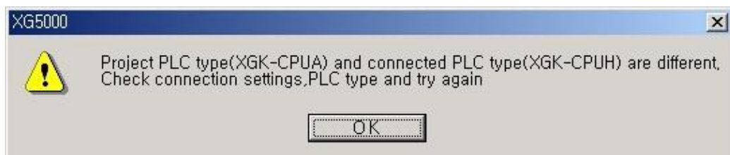
[Fig. 6.2.6] [CPU type is incorrect]
