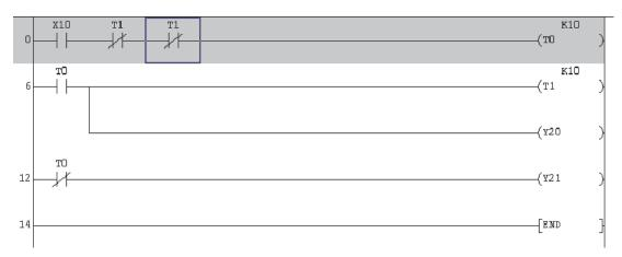
6 Press F4 to convert the addition of the normally closed X11.
