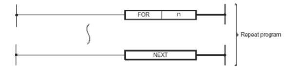
It is common practice to use a Conditional Jump (CJ) to bypass a FOR-NEXT loop if it is not required to be scanned. This will avoid scanning the loop when it is not required, thus minimising the overall program scan time.
