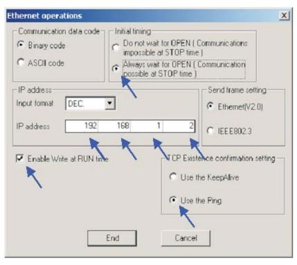
After the settings here are made, click *End* to return to the main network parameter setting window. Note that the *Operational settings* button has now changed to blue, indicating that changes have been made.
