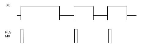
From the above waveforms, it can be seen that each time Input X0 operates, the Instruction PLS M0 will be executed and the normally open contact of M0 will momentarily close, hence causing the Counter C0 to be reset to zero.
