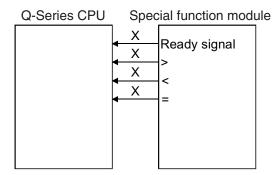
Xs used in the sequence program are signals generated and input by the special function module to the Q-Series CPU. They are used as contacts in the program, for example:
