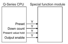
SET, RST and OUT-Y used in the sequence program are signals generated and output by the Q-Series CPU to the special function module. They are used as coils or contacts in the program.
