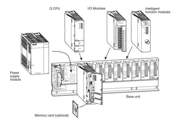
The CPU and modules are held in a base unit which has an internal bus connection for communication between the individual modules and the CPUs. The power supply module which supplies the voltage for the entire system is also installed on this base unit.
