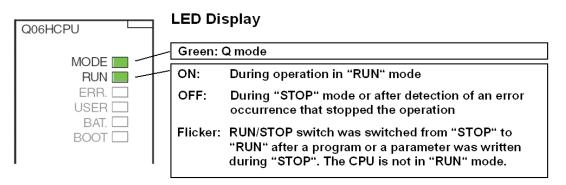
Procedure to switch a Q CPU from "STOP" to "RUN" after the program or parameters have been changed during "STOP":
