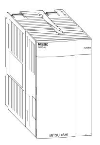
The power supply modules supply 5 V DC to each module on the base unit. Power supply modules with input voltages of 24 V DC or 240 V AC are available.
