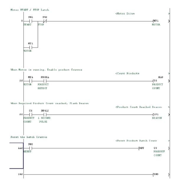
As can be seen, the display has replaced the Device Names with the Alias where appropriate.
