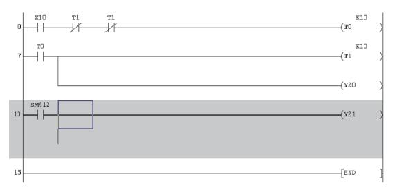
② Move the cursor down one line and press the "Output coil" button or press 7 on the keyboard. Enter C0 K10 and the display will be as follows:
