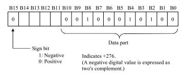
The above diagram shows an example of a 16-bit digital value written from the Q-Series CPU to the digital-to-analogue converter module. Set a digital value of -2048 to +2047 in 16-bit signed binary.
