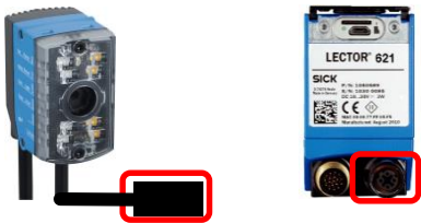
Profinet on P3: 4 pin, M12, D-coded
