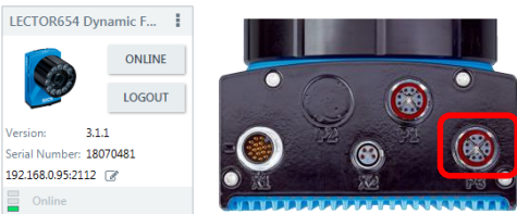
Profinet on P3: M12, 8-pin, X-coded
