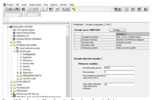
Figure 10-8 Example: TO configuration, "Encoder configuration" tab
