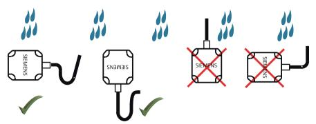
Figure 13-1 Permissible and impermissible cable routing when connecting in a damp environment
