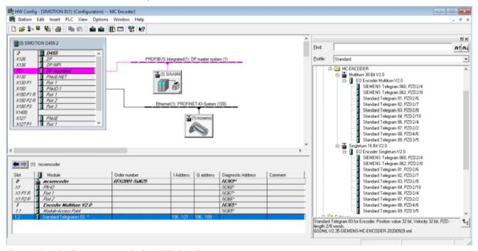
Figure 9-2 Setting up an encoder in a STEP 7 project
