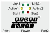
Figure 4-3 LED display - rear side of the encoder housing
