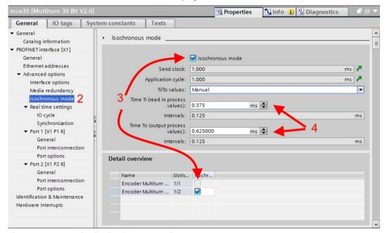
Figure 11-17 Activating isochronous mode
