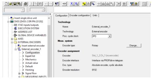
Figure 10-7 Example: TO configuration, "Configuration" tab
