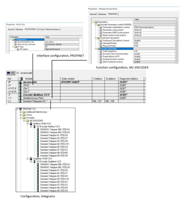
Figure 6-2 Example: Encoder access points for configuration and parameterization
