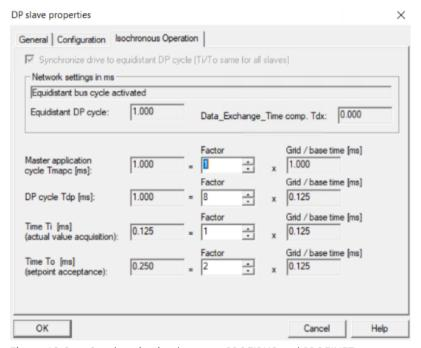
Figure 12-2 Synchronization between PROFIBUS and PROFINET
