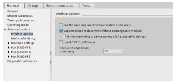
Figure 11-13 Allowing device replacement
