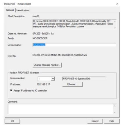
3. Define a device name and click on button "Ethernet" to define the encoder IP address.
