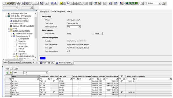
Figure 10-11 List of variables for cyclic encoder data in SIMOTION Scout
