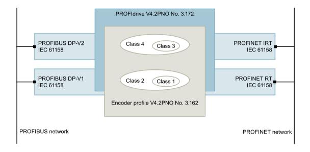
Figure 3-1 Overview of the documents relating to the standard and assignments to the individual technologies
