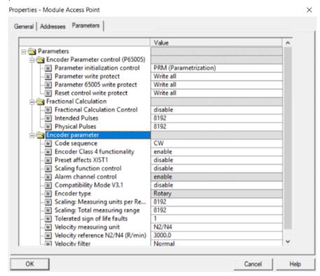
Figure 9-11 Setting encoder parameters
