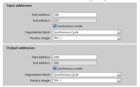
Figure 11-20 I/O addresses configured
