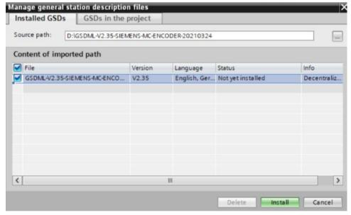
Figure 11-5 Installing GSDML
