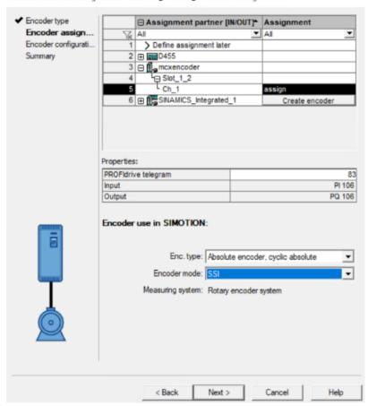
Figure 10-4 Assigning an encoder, configuring the type and mode
