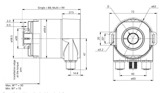
Figure 15-1 \*\* Insertion depth into the shaft
