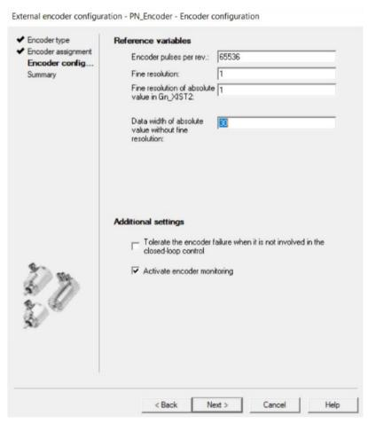
Figure 10-5 Configuring an encoder
