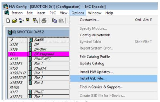
Figure 9-1 Installing the GSD file in STEP 7 HW Config
