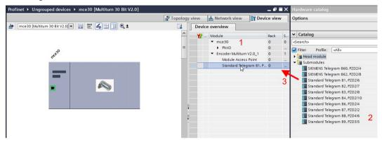
Figure 11-9 Inserting a telegram
