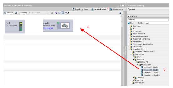
Figure 11-3 Inserting an encoder
