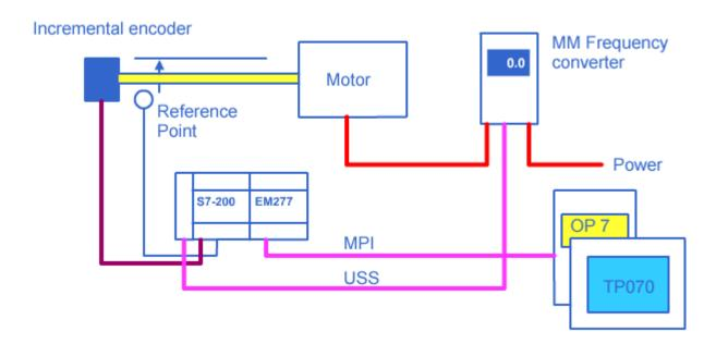
In this example, the encoder's reference point signal is not activated via an NO contact until the end of the path has been reached. This is necessary because the function of the high-speed counter cannot be changed while the controller is in RUN mode.
