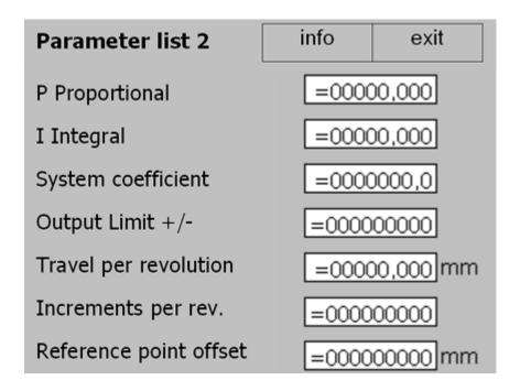
The system coefficient is a factor that depends on the overall configuration.
