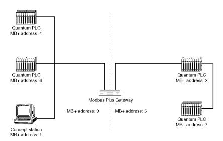
The address must be entered from the point of view of the receiving PLC to the sender, and thus begins at the first gateway or the next PLC. This depends on whether the sender and the receiver are located in the same Modbus Plus segment (no bridges/gateways) or whether the sender and the receiver are located in different segments (separated by one or more bridges/gateways).
