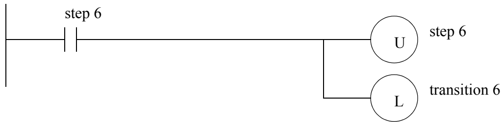
Figure 20.9 SFC Implemented in Ladder Logic
