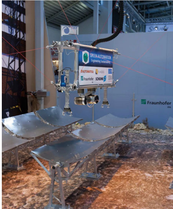
Fig. 2.9 Cable robot IPAnema 2 for large-scale handling of collector modules shown at Automatica 2010 trade fair, Munich, Germany
