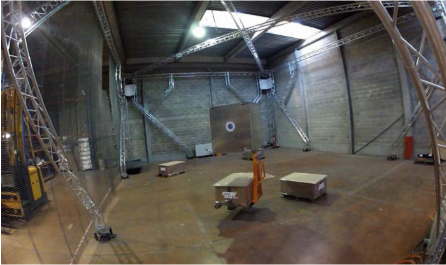
Fig. 9.17 CoGiRo: a large-dimension suspended cable-driven parallel robot with six degrees-of-freedom by LIRMM and TecNALIA. (Courtesy of LIRMM, Montpellier, France)
