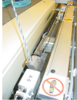
Linear actuation of the String-Man (Courtesy of Fraunhofer IPK, Berlin, Germany)
