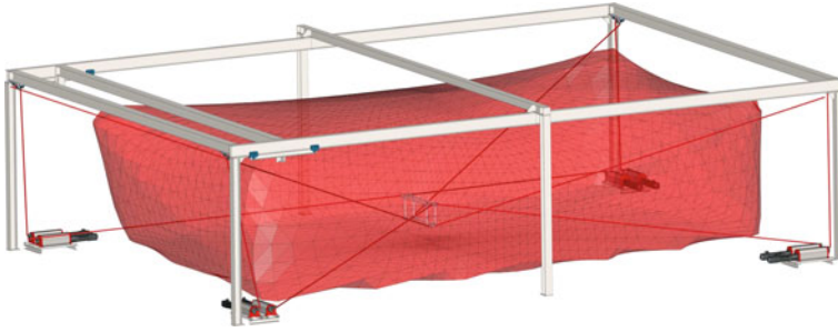
Fig. 8.8 Layout and workspace of the IPAnema 3 robot
