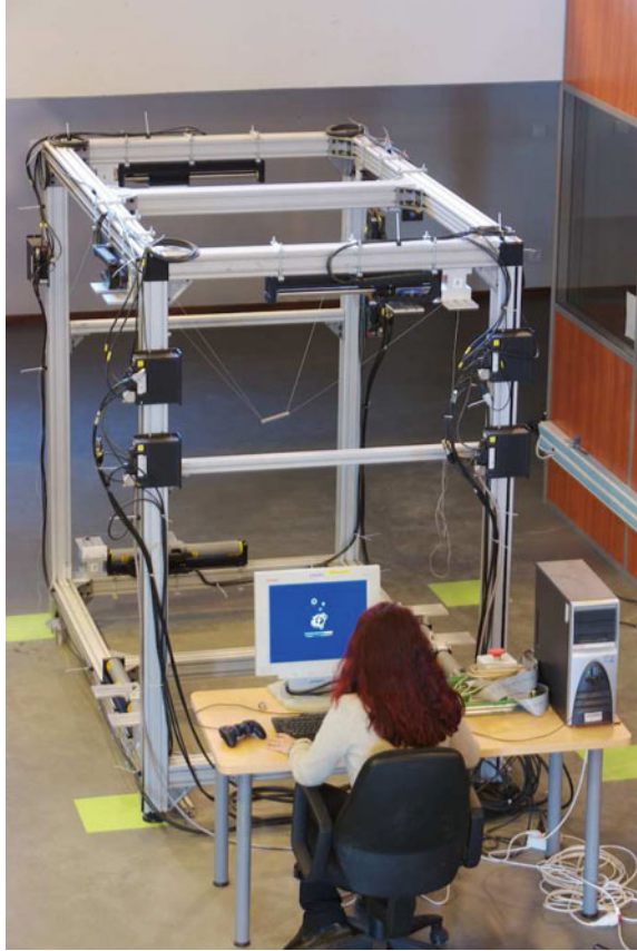
Fig. 2.16 The cable robots of the Marionet family for rehabilitation from Merlet (Courtesy of INRIA Sophia-Antipolis, France)
