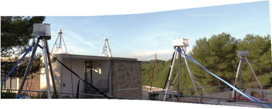
Fig. 2.23 The cable robots of the Marionet family for rehabilitation purpose and for rescue from Merlet (Courtesy of INRIA Sophia-Antipolis, France)
