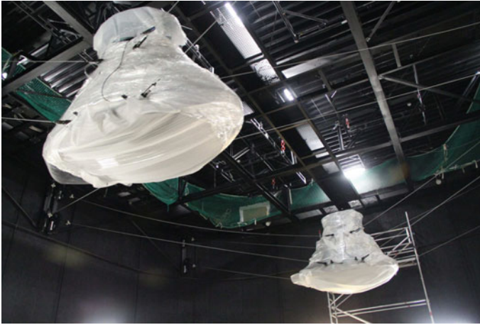
Fig. 9.13 Cable robots in transporting film during commissioning at the German Pavilion at EXPO 2015
