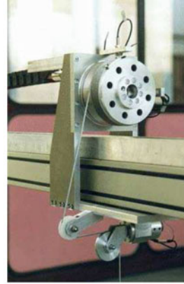
Cable winch with pulleys for guiding the cable. The second pulley is equipped with a rotation sensor to estimate the direction of the cable. (Courtesy of Chair of Mechanics, University of Rostock, Germany)
