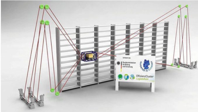
Fig. 2.12 The large-scale cable robots as storage retrieval machine CABLAR by University Duisburg-Essen (Courtesy of Chair of Mechatronics, University of Duisburg-Essen, Germany)
