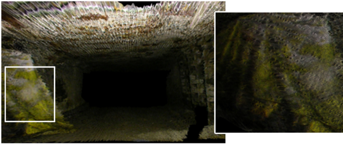
Fig. 4 Colorized 3D Reconstruction. Full scene (left) and mine curtain detail (inset and right).
