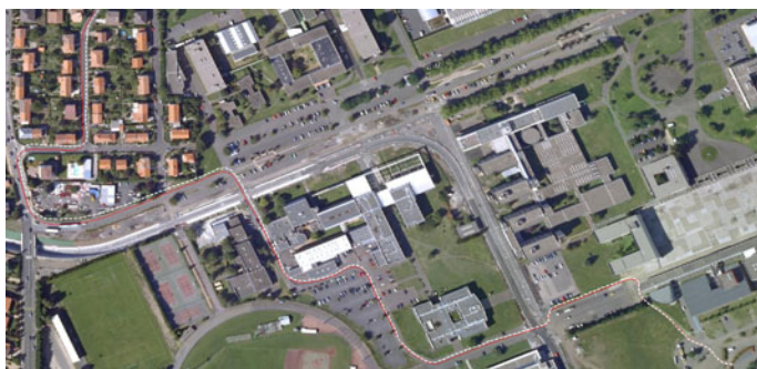
Fig. 2 Overlay of the estimated trajectory and the aerial image of Blaise Pascal University campus. The total traveled distance is around 1,135 m. The thin red line shows the trajectory of the vehicle measured with a centimetrically-precise GPS. The vehicle estimates are in thick white dashes.
