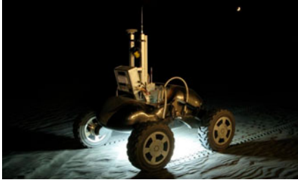
Fig. 1 The Scarab lunar rover. The glow beneath is from LED lighting for the optical flow sensor.
