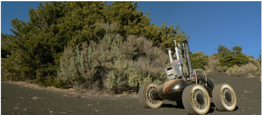
Fig. 4 Scarab, a four-wheeled prototype lunar prospector with an independent articulating chassis. In this configuration, the robot has exploited the articulating chassis to minimize roll of the body, thereby limiting exposure to tip over.
