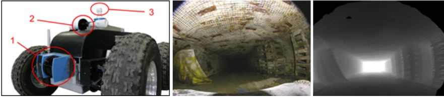
Fig. 1 (Left) Experimental setup with 1. LIDAR scanner, 2. Fisheye Camera, 3. Light Source. (Center) Raw fisheye imagery. (Right) Ground truth range image.
