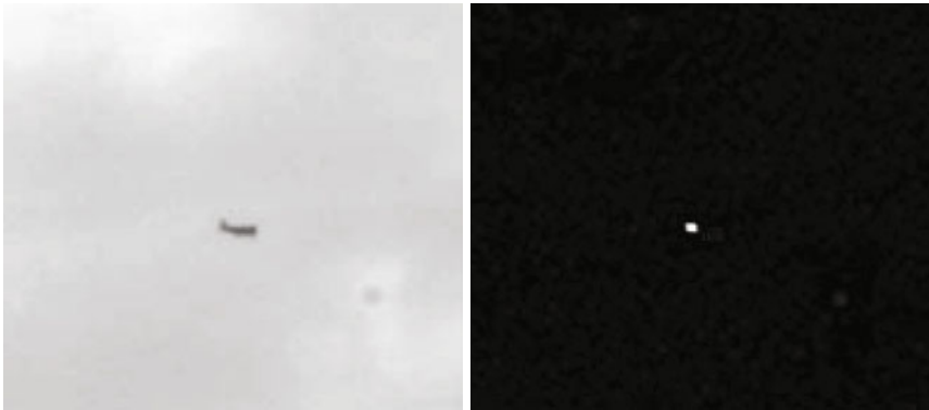
Fig. 3 The image on the left shows part of the image of the Piper Archer II at a range of 2.87 miles. The image on the right shows the result of the morphological operation of the left image in Stage 1 of the processing pipeline. The dark aircraft image shows up as bright white spot.
