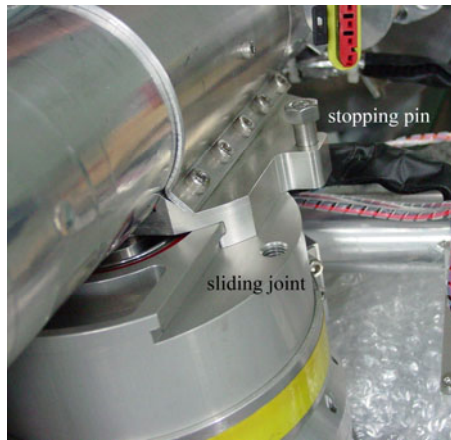
Fig. 4 Sliding joint for easy assembly.
