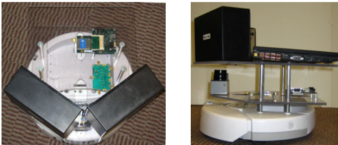
Fig. 1 Top and side profiles of AALS showing the integration of Hokuyo URG-04LX LIDAR, RFID reader, and on-board computing.
