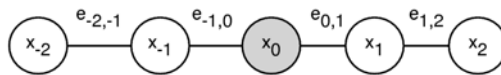
Fig. 2 A 1D chain of range nodes (a section of \mathbf{x} ) and the edges between neighbours. Considering x_0 , right extrapolation uses only nodes to the right and left extrapolation uses the two left hand nodes. Interpolation uses nodes x_{-1} and x_1 . The edges between nodes are a function of the difference in pixel appearance between adjacent range nodes (each range node is associated with a single pixel in the image).
