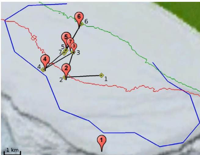
Fig. 4 Computed waypoints (yellow diamonds) and actual glider locations (red droplets). Image created by use of Google Earth.
