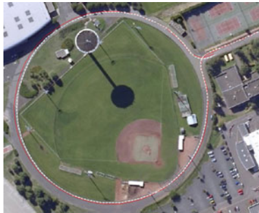
Fig. 5 The total traveled distance is around 700 m. The thin red line shows the trajectory of the vehicle measured with a centimetrically-precise GPS. The vehicle estimates after the loop closing are in thick white dashes.
