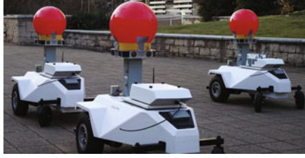
Fig. 1 Three robots used for experimental evaluation of the proposed leap-frog localization strategy.
