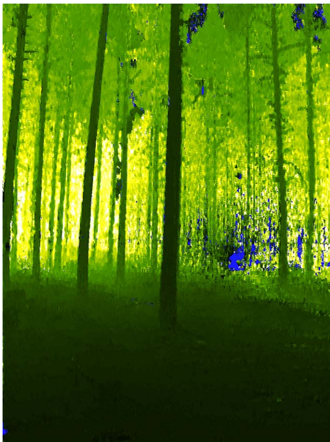
Fig. 4 A structure estimate for an instantaneous moment in a forest. Color brightness indicates the depth; the brighter, the further away.
