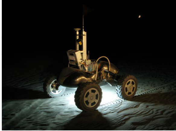
Fig. 5 Scarab navigating in darkness. Laser scanner perceives terrain ahead and an underbody optical velocity sensor detects slip.
