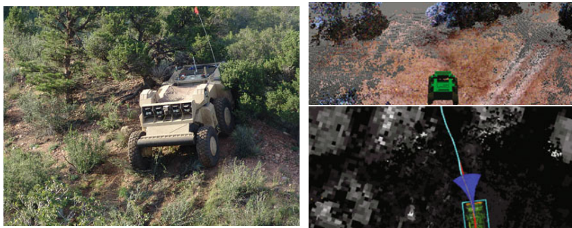
Fig. 1 Crusher (Left) is capable of autonomous navigation through complex outdoor terrain. Perceptual data (Top Right) are converted to costs (Bottom Right) for use by the planning system.
