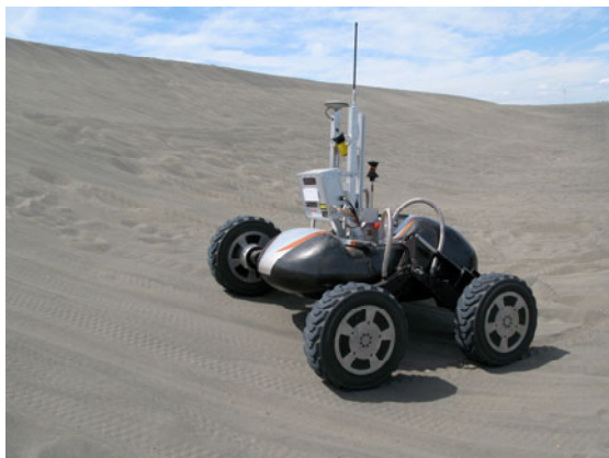
Fig. 1 Scarab lunar rover prototype on unconsolidated sandy soil in eastern Washington
