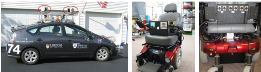
Fig. 1 Development Platforms. (Left) Vehicle used for data acquisition. Ben integrates an OXTS RT-3050 and a pair of vertically scanning Sick LMS291-S14 LIDARs (circled red). (Center-Right) Our smart-chair platform integrates LIDAR, vision, GPS, and odometry sensors. Its computer interface and on-board power distribution enable a range of sensors and accessories to be quickly integrated for prototyping purposes.
