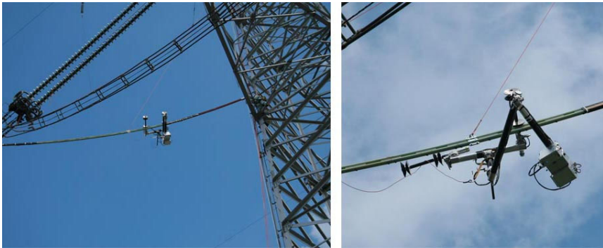
Fig. 11 Expliner moving on loading pipe (left) and performing an automated motion.
