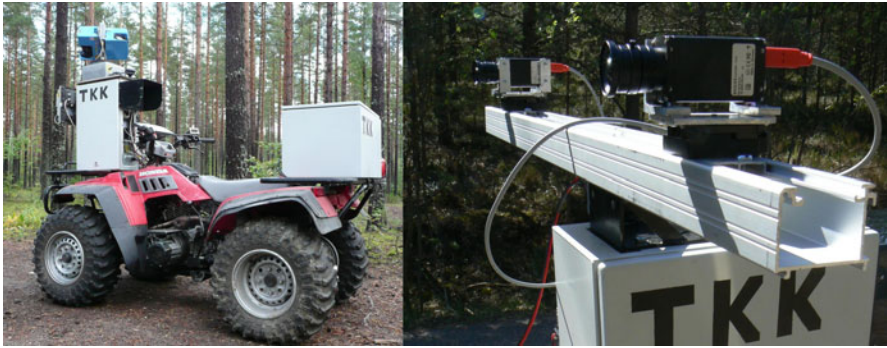
Fig. 2 ATV platform with 3D scanner measurement equipment on the left and stereo camera pair on the right.
