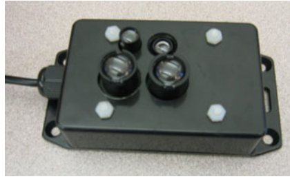
Fig. 2 The optical sensor used on Scarab, in a custom ruggedized enclosure.
