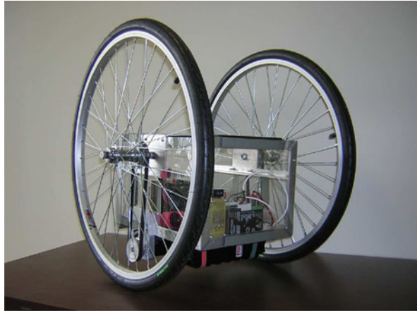
Fig. 1.14 QUASIMORO, a quasiholonomic mobile robot
